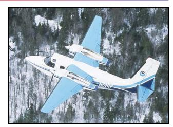
The NOHRSC uses two low-flying aircraft to make airborne snow water equivalent measurements across the U.S. including Alaska. Each winter airborne snow measurements are made from a network of over 2,200 flight lines covering portions of 31 states and 7 Canadian provinces. The data are reported in near real-time to the NOHRSC office in Minneapolis and distributed to other NWS offices and the NOHRSC web site within an hour after the survey aircraft land each evening.
