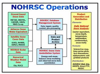
The NOHRSC continuously ingests a variety of ground-based, airborne, satellite, radar, and numerical weather model data from multiple sources across the country. The data are managed in a database system and processed by the SNOW Data Assimilation System (SNODAS). Products are generated and distributed to end users across the country over the NOHRSC web site and the NWS computer network.
