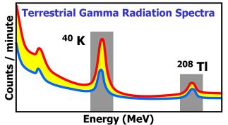
Natural, terrestrial gamma radiation emitted from the upper 8 inches of soil is used to infer snow water equivalent on the ground. A one-time background radiation spectrum (red) is collected with no snow on the ground. The water in the snowpack blocks the radiation signal. The difference (yellow) between the background (red) and the over-snow radiation spectra (blue) provide the ability to measure the snow water equivalent on the ground with an error of less than one cm of water equivalent.
