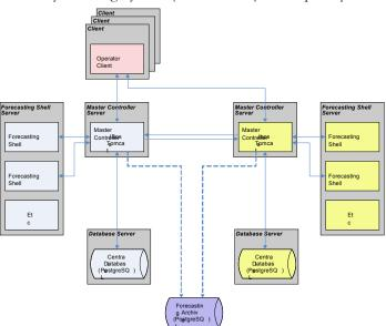
**Figure 5.3.** The major components of CHPS are the Database Server, Master Controller, Forecasting Shell Server, and Operator Client. The left systems (grey) are the primary systems, and the right (yellow) are standby systems.
