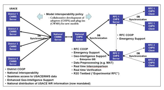
**Figure 5.3.** Straw diagram showing system interoperability and database synchronization implementation for NWS CHPS and USACE CWMS. By linking between regional nodes and to a central national node, a variety of benefits can be realized (bullets). Although exceptions are still anticipated, USACE is in the process of migrating to two national server centers to serve as the principal hubs for external network communications, making this approach essential for NWS-USACE communications.
