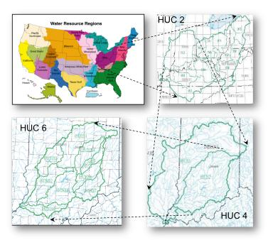
**Figure 6.4.** Twenty-one USGS Water Resource Regions (upper left). Within each region, watersheds are nested hierarchically and identified by two, then four, then six-digit hydrologic unit codes (HUC).
