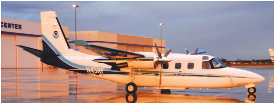
The NOHRSC airborne survey aircraft uses remote sensing of gamma radiation
